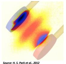
Carbon plasma streams ablating off paddles hit by laser beams and colliding with each other Multifluid phenomena that we want to model
